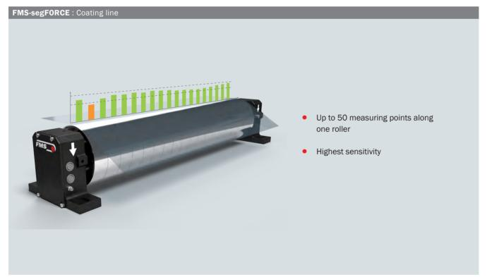
Fully equipped segmented measuring roller with brackets (type P pillow block) for universal mounting on the machine frame. Only a 24 (18 to 38) VDC power supply and a compressed air connection are required. Data connection is realized with an RJ-45 socket.
