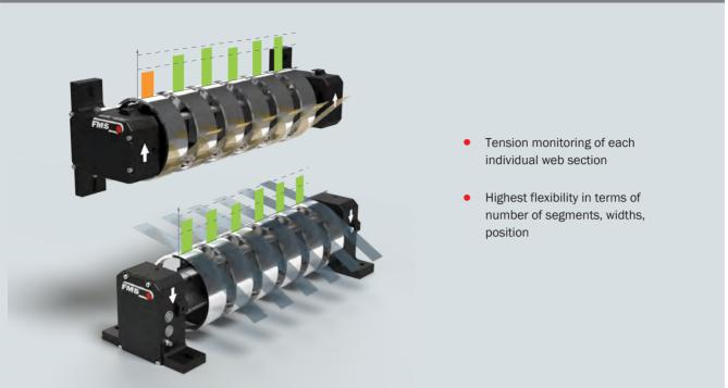
Schematic of two measuring rollers in the slitter / rewinder. The offset of the individual segments from the lower to the upper measuring roller can be seen clearly. Smallest differences in tension between the individual web sections quickly become visible. The sophisticated design allows all types of wrap angles to be covered. Flexible segment widths and freely adjustable distances between the segments make it possible to configure the measuring rollers for a wide variety of slitting widths.
