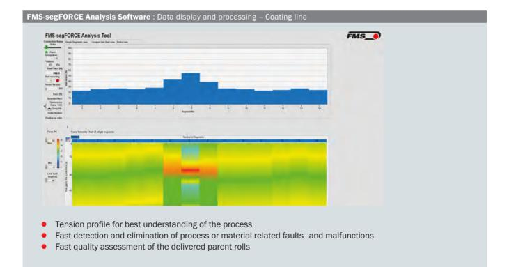
Top: Measuring values from each individual segment. Bottom: Waterfall diagram of a baggy web. This defect pattern can only be detected with a segmented tension roller.
